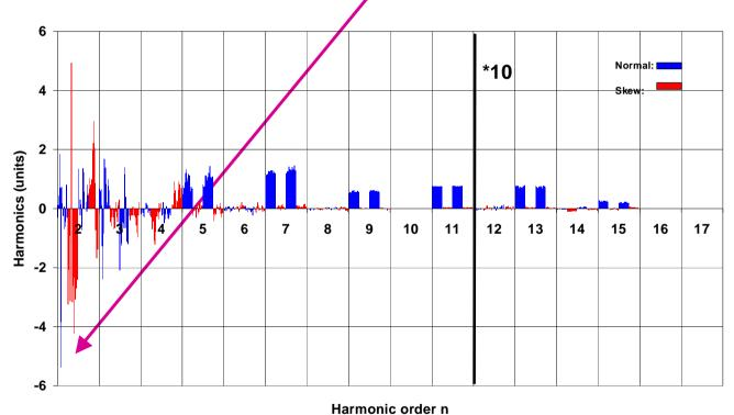
HCMB\_\_A001-01000027 - Collared coils - Harmonics along the axis
