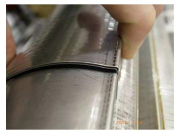
Decollared, it has been found that it was erroneously assembled with two coil protection sheets (0.5 mm more !) on a 1-m section
