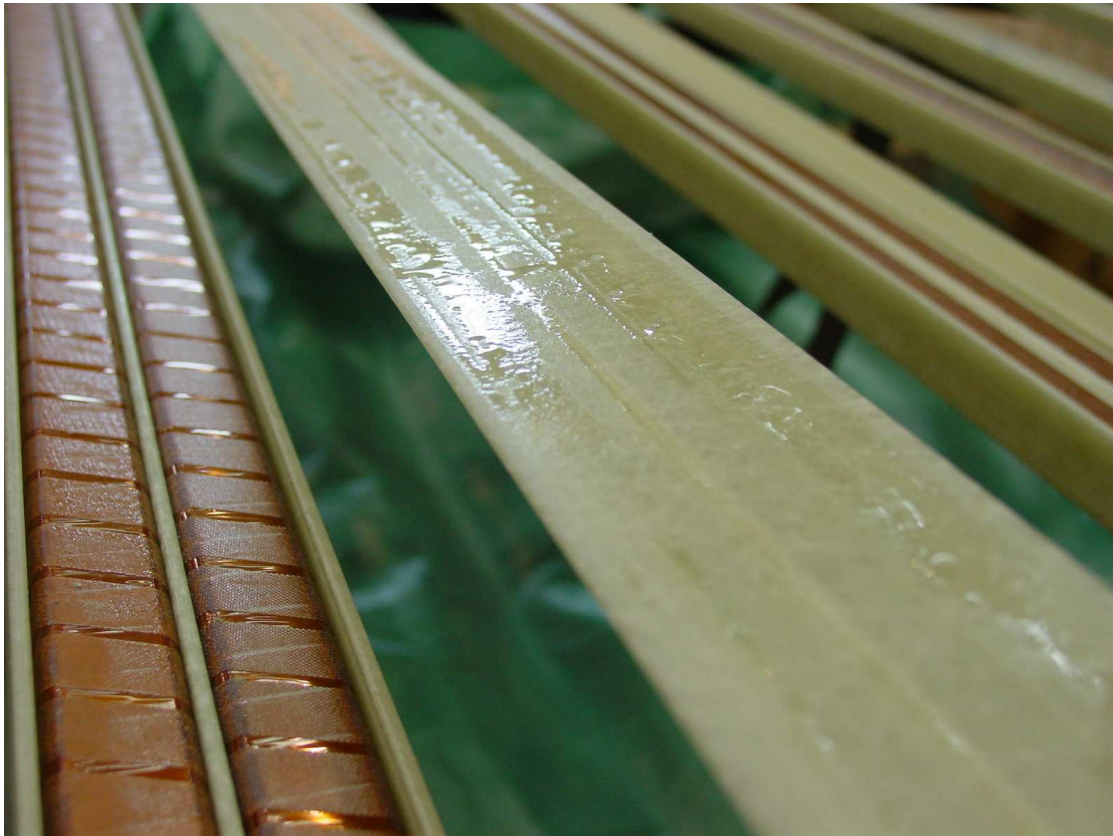
Fig. 9: Water found inside after lid removal
