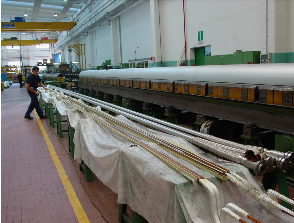
Fig. 13: Bus-bars opening and drying
