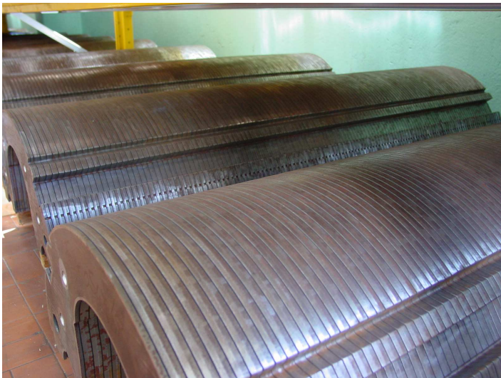
Cleaned lamination just before half yoke assembly
