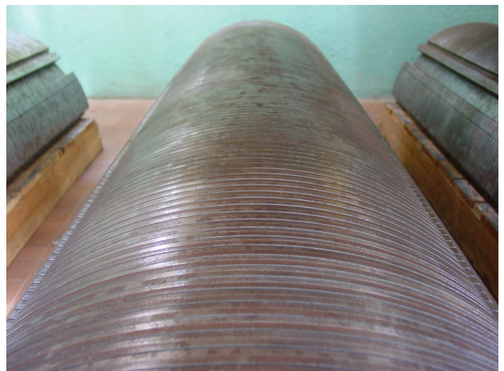
Detail of cleaned lamination
