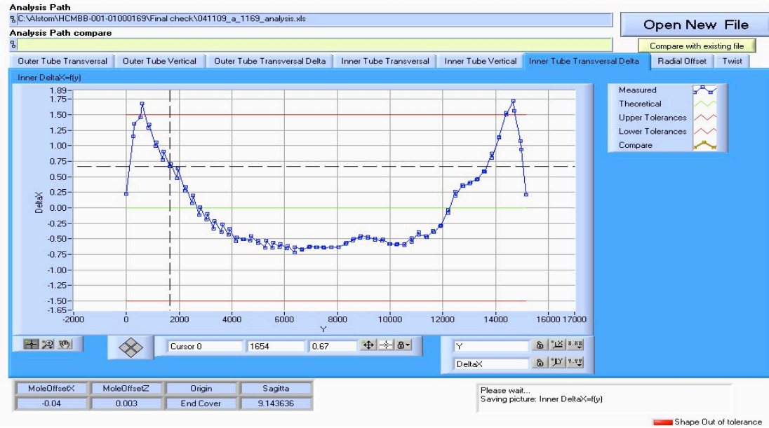
Figure 3. Shape error on cold mass 1169
