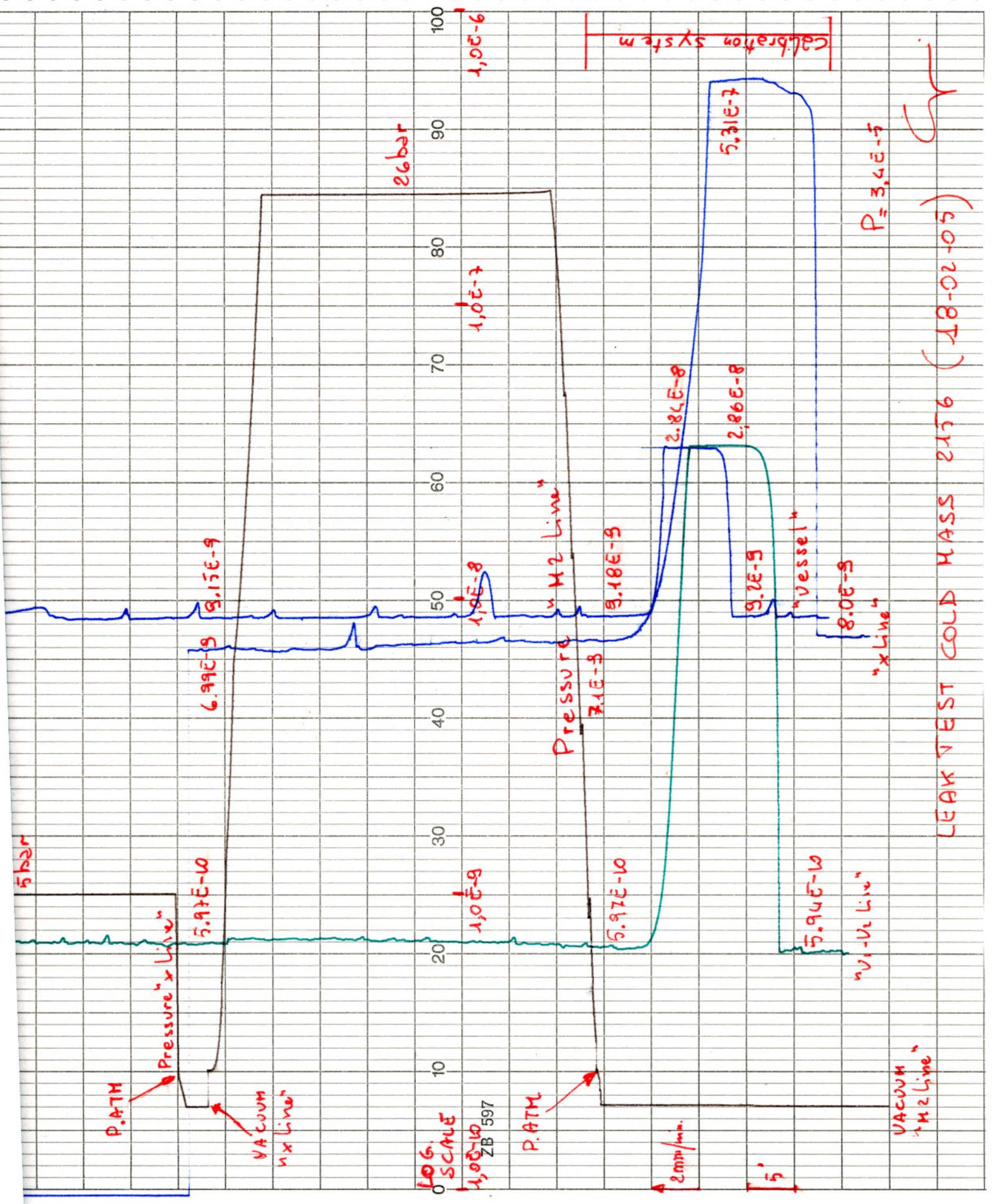
LEAK TEST COLD MASS 2176 (18-02-05)
