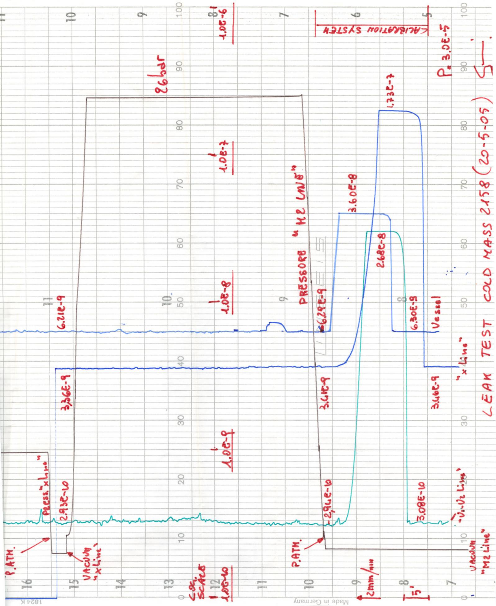
LEAK TEST COLD MASS 2158 (20-5-05)
