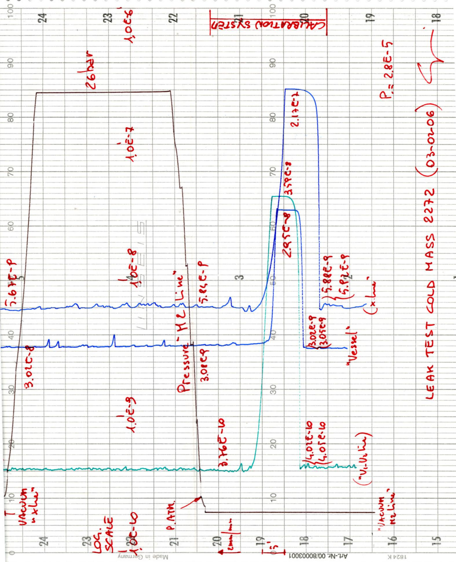
LEAK TEST COLD MASS 2272 (03-02-06)
