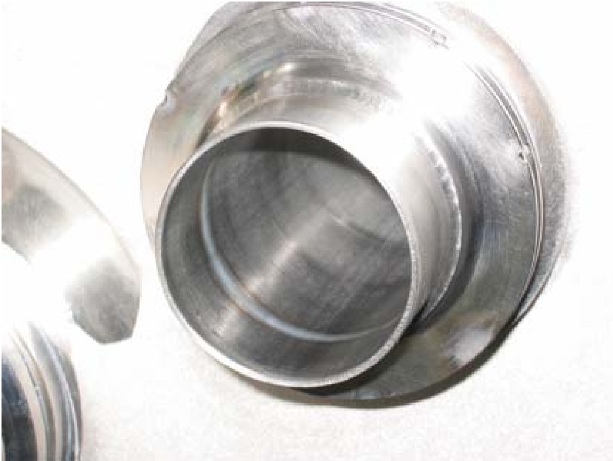
Figure 3 : C.b.t. to collerette weld, free of defect
