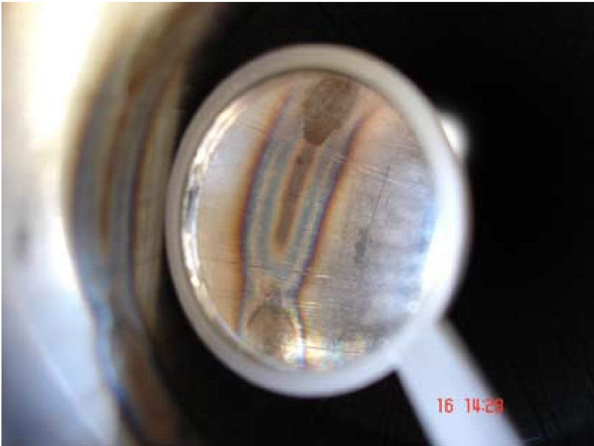
Figure 21 : Scaled surface – Defect N°613
