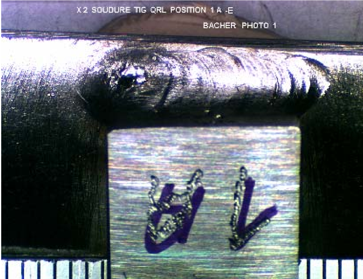
Figure 14 : End crater pipe – Defect N°2025
