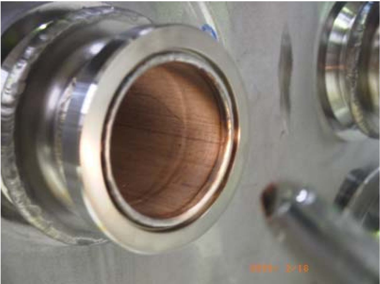
Figure 2 : C.b.t. to collerette weld, free of defect
