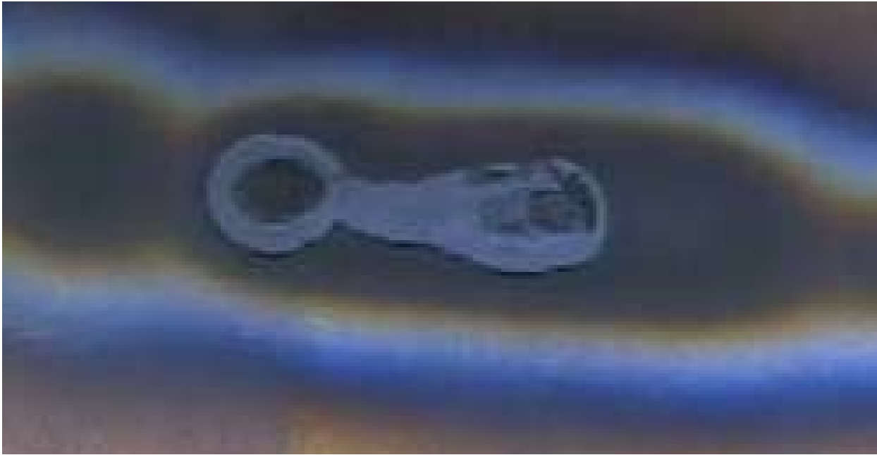
Figure 13 : Root porosity – Defect N°516
