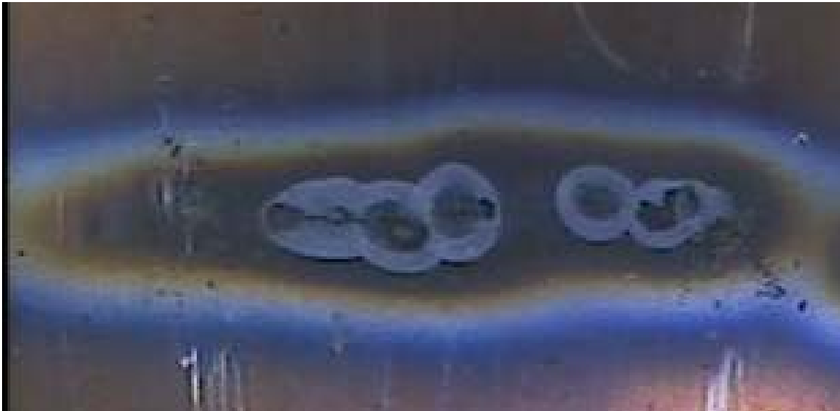
Figure 12 : Root porosity – Defect N°516
