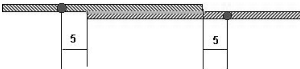
Figure B10.1 Measurement of the layer jump resistance: position of the voltage pickups (dim. in mm)
