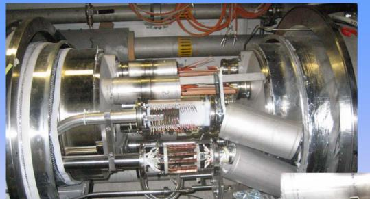
600A line (cabling boards completed, before connection)
