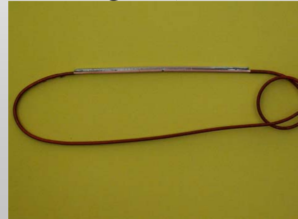
If there is not enough conductor .. double brazing. Each superposition length >50mm
