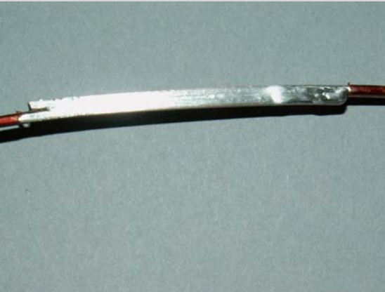
Simple brazing. Superposition length >50mm
