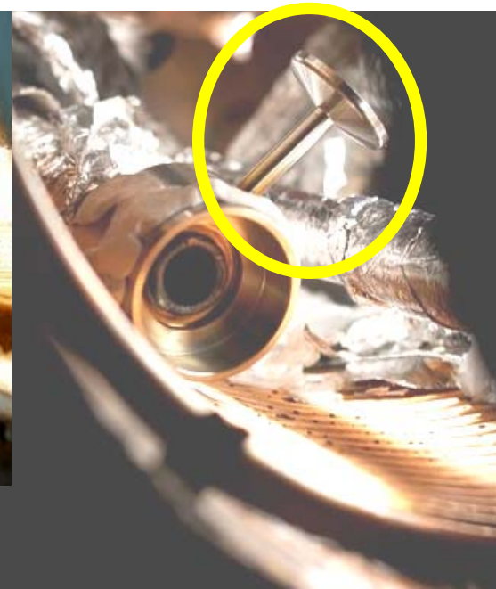
Homemade leaktest "clams shell"
