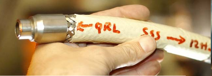
Leaking metal hose
