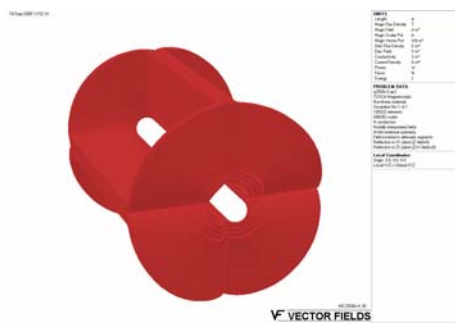
Fig. 6 3D model of the coil. Main coil as well as corrector coil are saddle-shaped.
