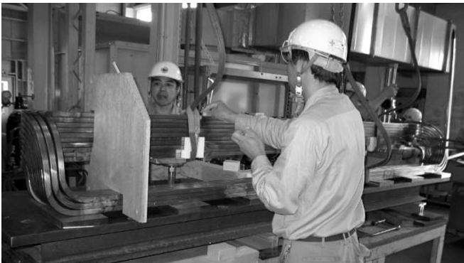
Fig. 3, One quadrant of Q350 (QC2) coil made of MIC at the final inspection. Coil dimensions were carefully checked by using the standard plate referring to the existing iron yoke of QC2.
