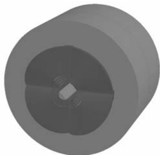
Fig. 5. 3D design of the quadrupole PQ 11 using the direct cooled cable MIC 2500A-H.
