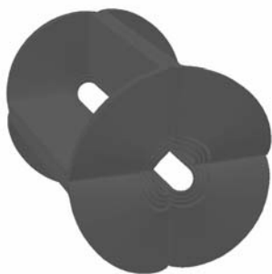
Fig. 6. 3D model of the coil. Main coil as well as corrector coil are saddle-shaped.
