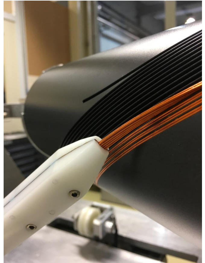
Fig. 59: Tooling allowing to wind ten strands in one go.
