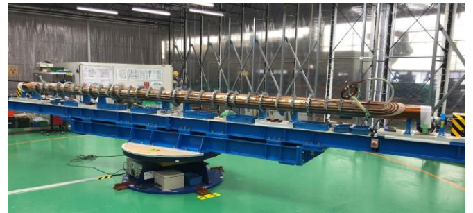
Fig. 36: Winding of the coil of the D1 prototype.
